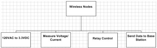
Figure 22: Level 1 Tier "Wireless Nodes" and Its Corresponding Level 2 Structures
