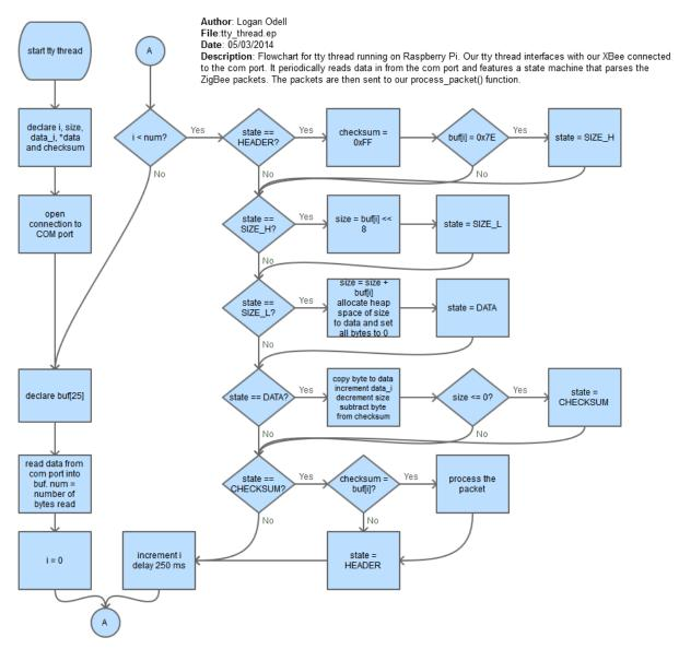
Figure 48: Flowchart for TTY Thread
