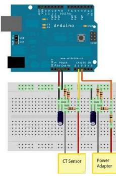
Figure 52: Energy Measurement Circuit
