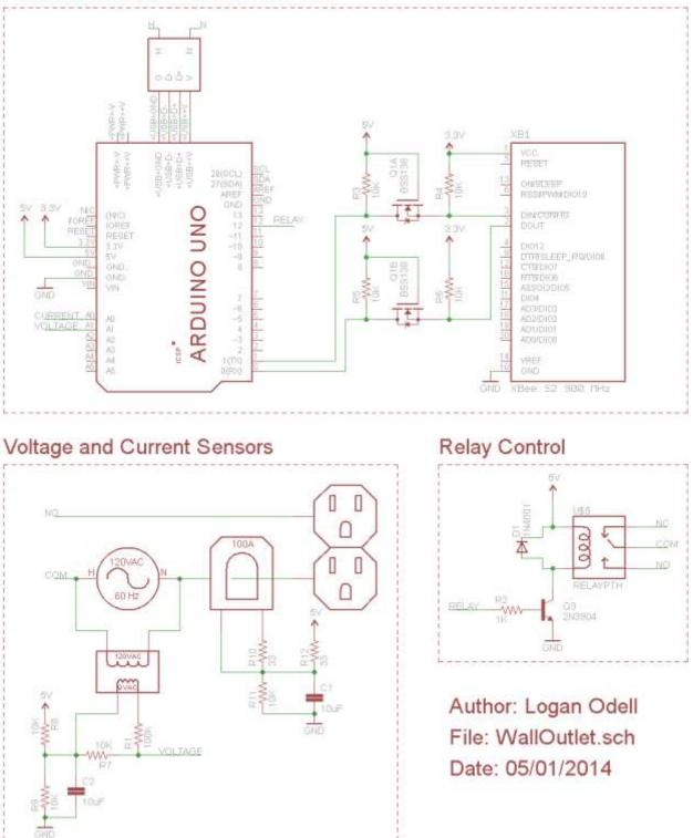
Figure 41: Schematic For Wall Outlet Node Device
