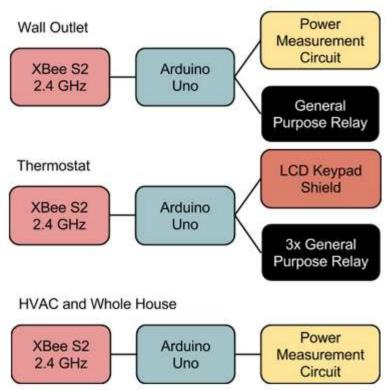
Figure 40: Node Device Block Diagrams
