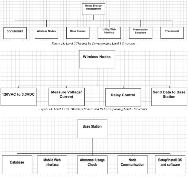
Figure 15: Level 1 Tier "Base Station" and Its Corresponding Level 2 Structures
