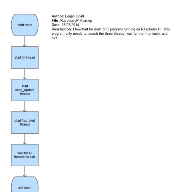
Figure 47: Flowchart For Raspberry Pi Main Function
